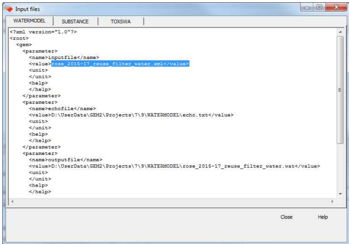
Figure A6. Screenshot of the input file of the WATERSTREAM model. The input file name refers to the combination of reference crop- emission period and whether or not the filter water is reused.
