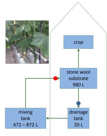
Schematic overview of the pilot scale greenhouse (120 m<sup>2</sup>). Substances dimethomorph, fluopyram and imidacloprid were applied with the nutrient solution to a standing cucumber crop with the nutrient solution. Samples were taken from water flowing into • and out of • the substrate. The mixing tank served as water reservoir as well. Fresh water (400 L) was added when the water content of the mixing tank dropped below 472 L.
