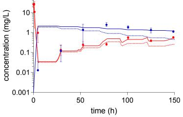
Fluopyram concentrations in the recirculating water in the system. Red: into, blue: out of the stone wool. Dots: measurements, lines: simulations. For comparison, the dotted lines give the results for TSCF = 1, clearly to high a value for fluopyram.
